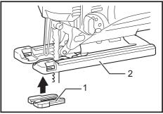
■ 1. Anti-splintering device 2. Aluminum base
