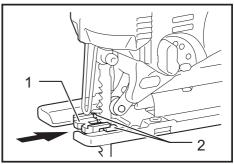
▶ 1. Anti-splintering device 2. Protrusions
