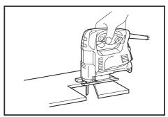
To trim edges or make dimensional adjustments, run the blade lightly along the cut edges.
